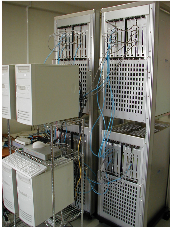
Fig. 7. The 32-board, 32-Tflops GRAPE-6 system with its host computer. The host is a cluster of 4 PCs with 1.7GHz Intel P4 processors connected by 100Mb Ethernet.
